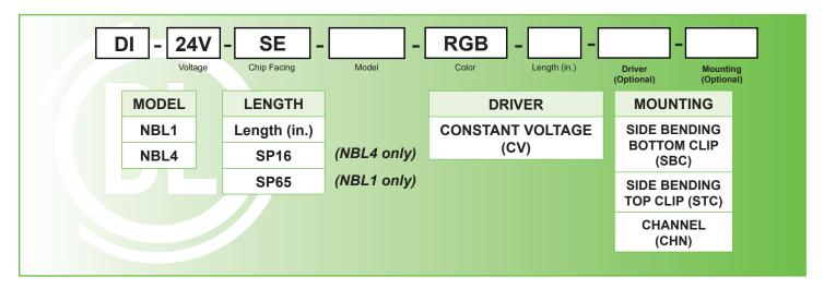
Example: DI-24V-SE-NBL4-RGB-16-CV-SBC = Diode LED, 24V NEON BLAZE<sup>TM</sup>, 4.44 w/ft. RGB, 16.4' long, 96" Lead Wire, and with a Constant Voltage Driver, and Side Bending Bottom Clips.
